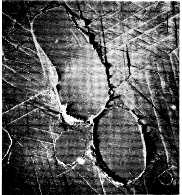
FIGURE 8. Cracking at carbide/matrix interfaces.
